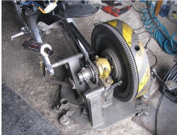
Figure 10 Measurement of experimental model on power brake
