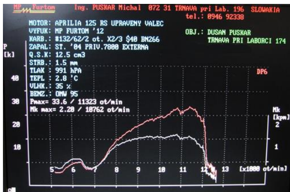
Figure 13 Performance and torque of the modified engine
